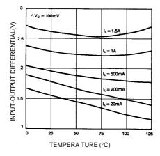
Figure 3. Dropout Voltage
