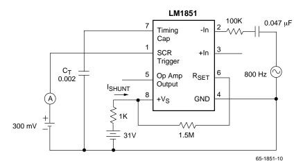
Figure 9. Normal Fault Sensitivity Test Circuit
