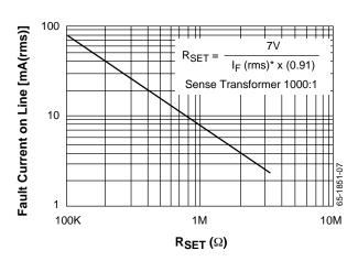
Figure 5. Normal Fault Current Threshold vs. RSET
