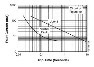
Figure 4. Average Trip Time vs. Fault Current
