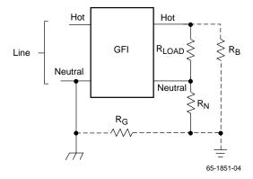
Figure 3. Normal Fault Plus Grounded Neutral Fault
