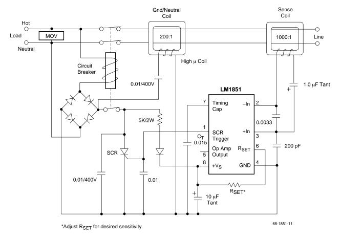
Figure 10. 120 Hz Neutral Transformer Application
