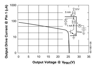
Figure 6. Output Drive Current vs. Output Voltage
