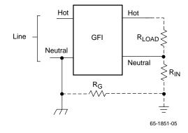
Figure 2. Grounded Neutral Fault
