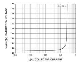
Figure 2. Collector-Emitter Saturation Voltage
