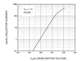
Figure 5. Base-Emitter On Voltage
