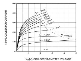
Figure 1. Static Characteristic
