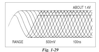
RF (eye pattern) waveform at DVD disc TK-47 board CN005 pin 26
