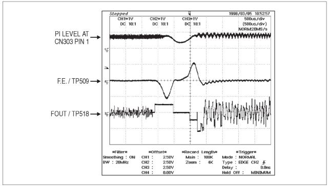
Fig. 1-36 Focus jump from layer 0 to layer 1
