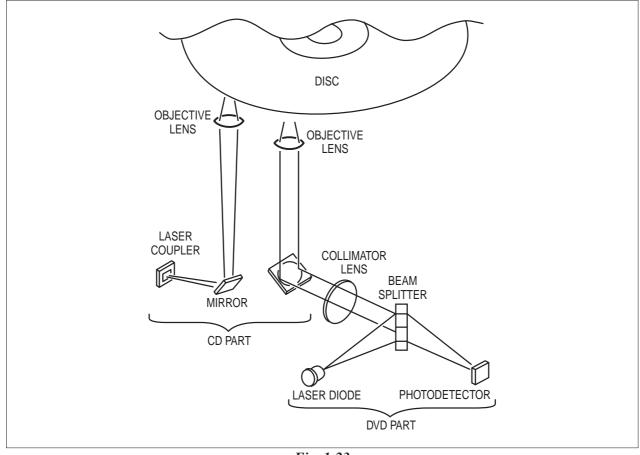
Fig. 1-23 DVD optical systems built in one OPU
