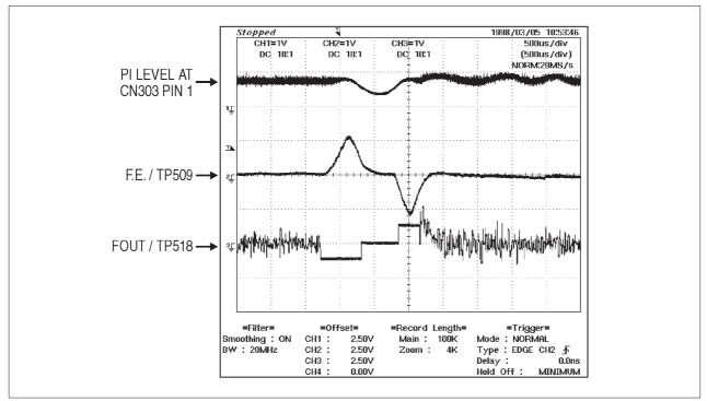
Fig. 1-37 Focus jump from layer 1 to layer 0
