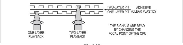
Fig. 1-35 2-layer disc readout method
