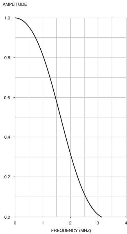
Figure 9.26. Typical 1.3 MHz Lowpass Digital Filter Characteristics.
