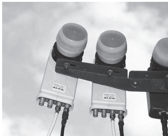
FIGURE 9.25 Quattro Universal LNBs have four outputs, like Quattro LNBs.
