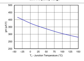
Figure 8. EA Transconductance vs Junction Temperature
