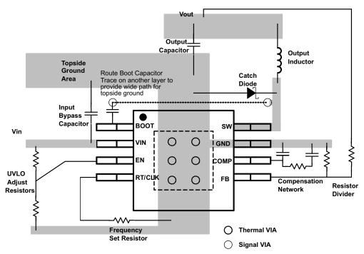
Figure 57. PCB Layout Example
