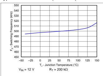
Figure 5. Switching Frequency vs Junction Temperature
