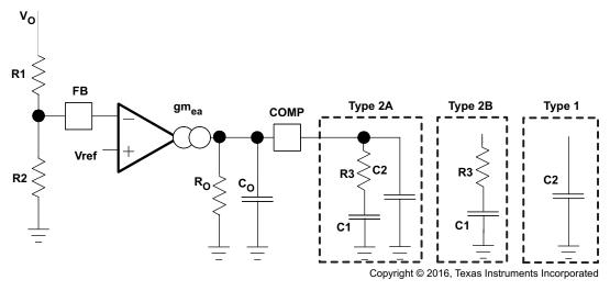
Figure 30. Types of Frequency Compensation
