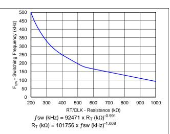
Figure 6. Switching Frequency vs RT/CLK Resistance
