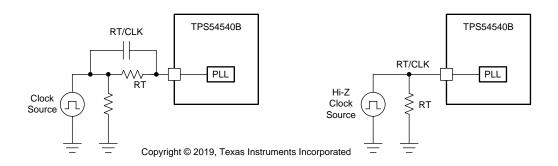
Figure 24. Synchronizing to a System Clock
