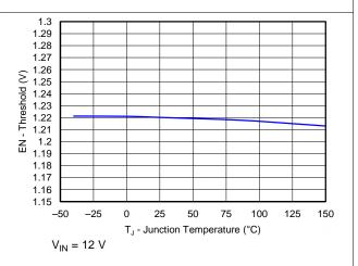
Figure 10. EN Pin Voltage vs Junction Temperature
