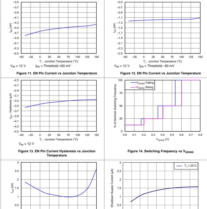
Figure 15. Shutdown Supply Current vs Junction **Temperature**
