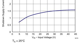
Figure 16. Shutdown Supply Current vs Input Voltage ( $V_{IN}$ )
