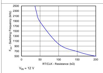
Figure 7. Switching Frequency vs RT/CLK Resistance
