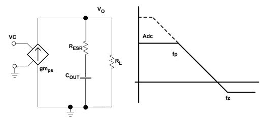
Figure 29. Simple Small Signal Model and Frequency Response for Peak-Current-Mode Control
