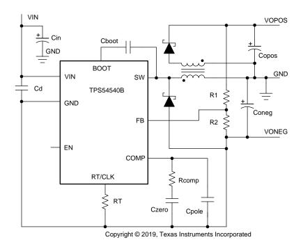
Figure 56. TPS54540B Split-Rail Power Supply
