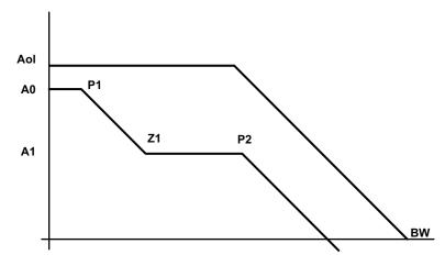
Figure 31. Frequency Response of the Type 2A and Type 2B Frequency Compensation
