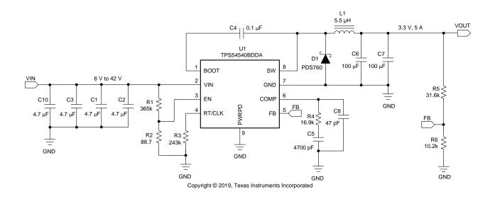
Figure 32. 3.3 V Output TPS54540B Design Example
