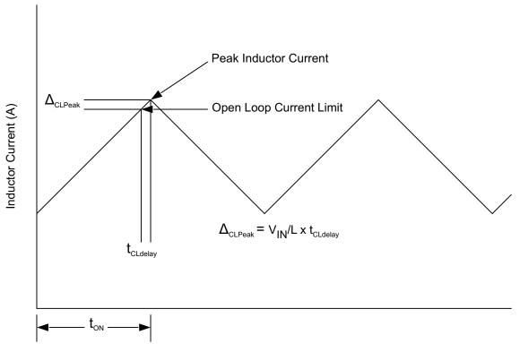
Figure 23. Current Limit Delay
