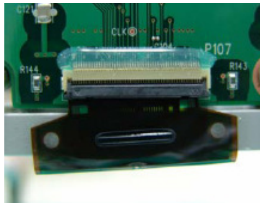
< metal particle between the electrode >
