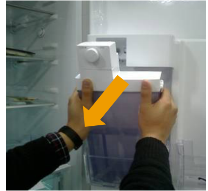
Remove the water tank.
