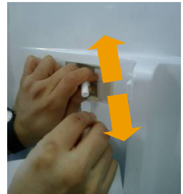
Pull out each other and Disconnect the tubes.
