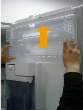
Remove the basket over the case pump.
