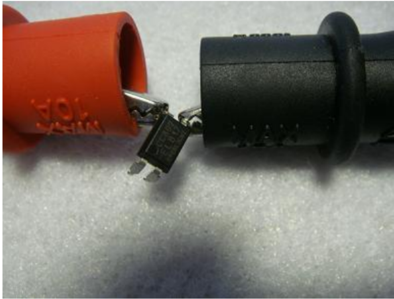
Attach test leads to the emitter and collector pins, polarity does not matter.
