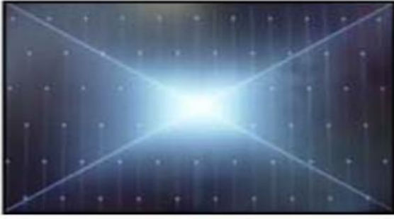
Solder defect, Short/Crack
