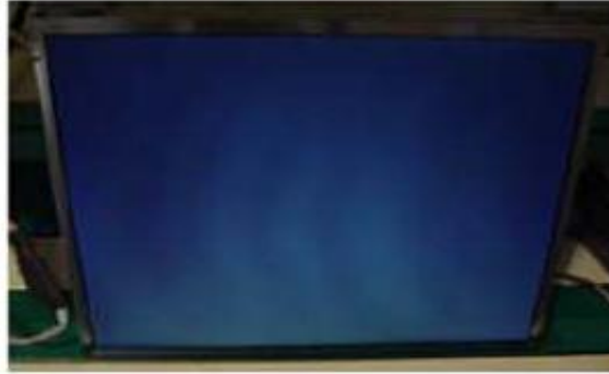
Panel Mura, Light leakage
