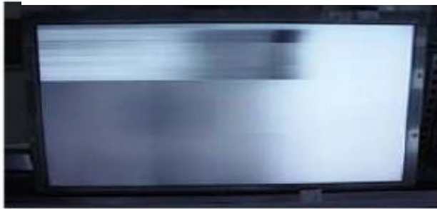
Horizontal Block Gate TAB IC Defect
