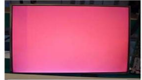
Vertical Block Source TAB IC Defect
