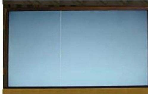
Vertical Line Source TAB IC Defect
