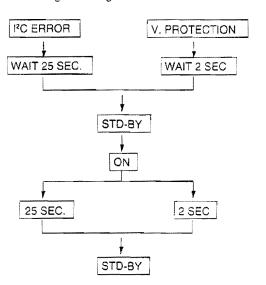
In the case of more than one error in parallel, the blinking error shows max priority according to the error number (e.g. error 2 and error 5 appear together, then LED,s show error 2).
