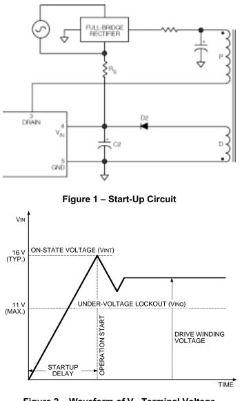
Figure 2 – Waveform of V<sub>IN</sub> Terminal Voltage at Startup
