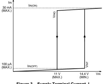
Figure 3 – Supply Terminal Current,  $I_{IN}$
